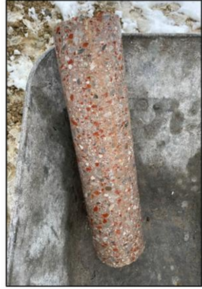
Fig. 13: Drill core with mixed recycled aggregate
