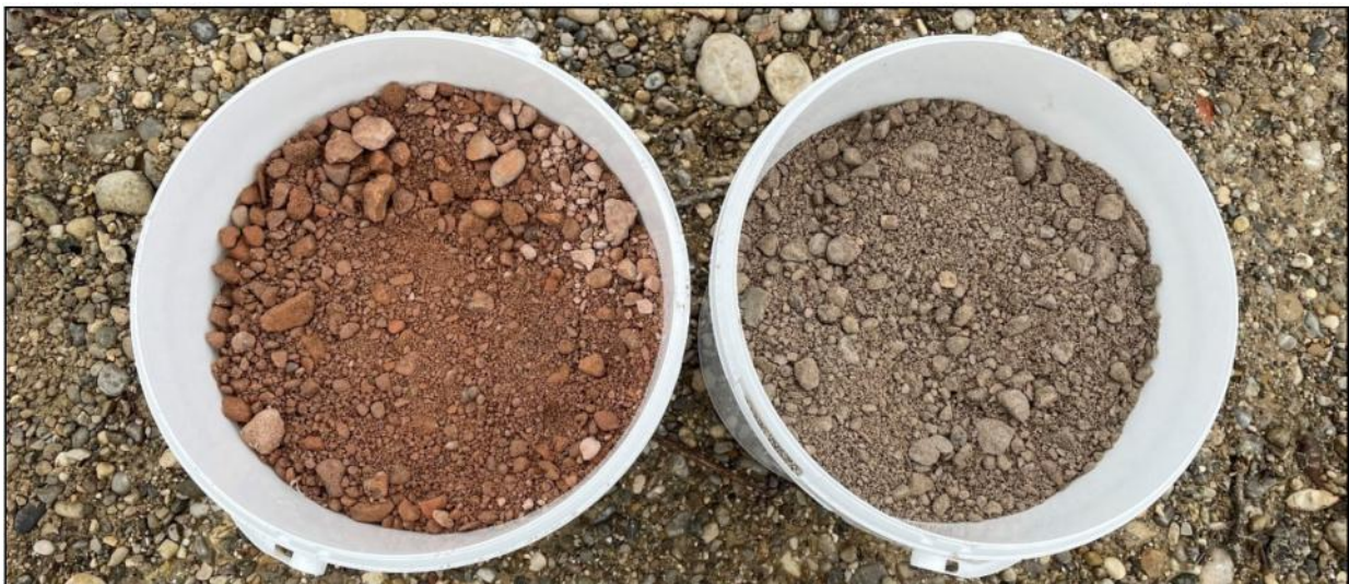
Fig.1: Mixed recycled aggregate (left) and concrete recycled aggregate (right)
