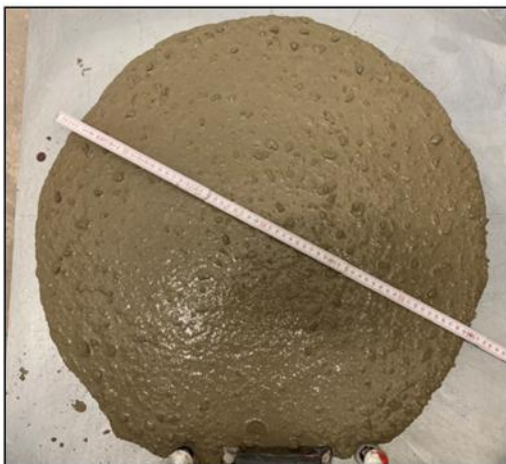
Fig. 8: Examination of the slump flow
